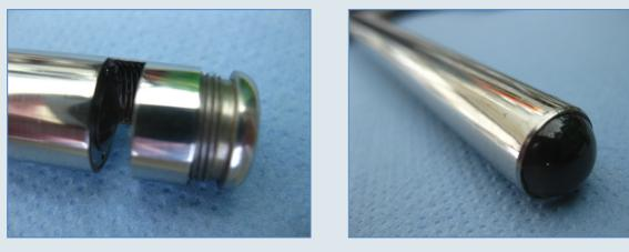
NIR transflectance probe with variable pathlength for liquid samples (up left); NIR diffuse reflectance probe for solid samples (up right).
