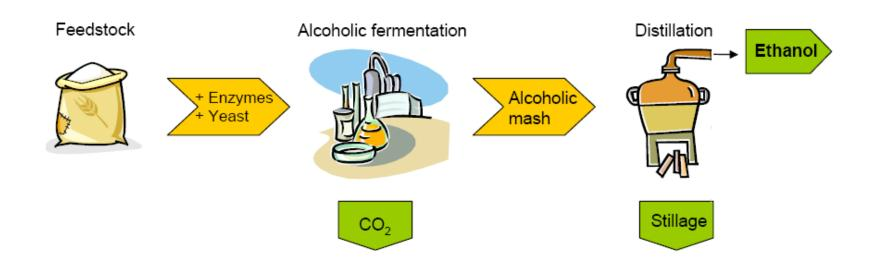
Wheat/rye/corn  $\rightarrow$  enzymatic pretreatment  $\rightarrow$  enzymatic starch degradation  $\rightarrow$  fermentation by yeast  $\rightarrow$  ethanol containing **mash**  $\rightarrow$  separate ethanol by distillation  $\rightarrow$  **stillage** remains as residue
