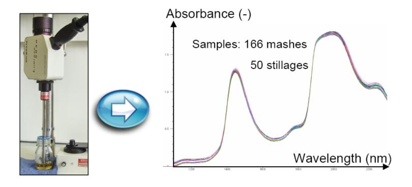
1100-2300 nm at 5 nm intervals, AOTF-NIR spectrometer *Brimrose Luminar 5030*, fiber-optic transflectance probe. 1<sup>st</sup> derivative spectra contain 235 *x*-variables; variable reduction to 15 (specific variables for each compound) by a Genetic Algorithm (GA) [2,3].
