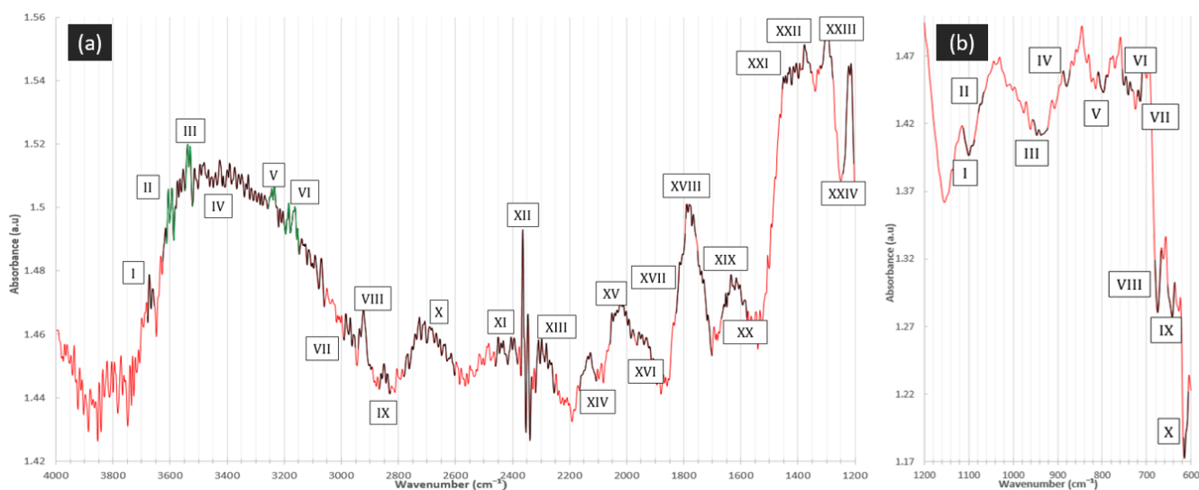
Figure 4.11: Reststrahlen bands (a) and absorption bands (b) of the spectrum number 13 with the roman number corresponding to each peak assigned in the table 4.2 and 4.3.
